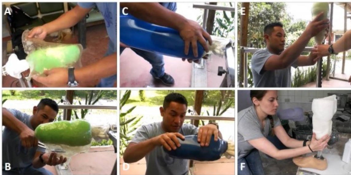
Figure 4. Fabrication method. A – Drape-molding thermoplastic, B – Trimming excess material (can be re-used), C – Applying global compression, D – Applying localized compression, E – Adjusting alignment of proximal socket-pylon adapter, F – Adjusting overall alignment.
